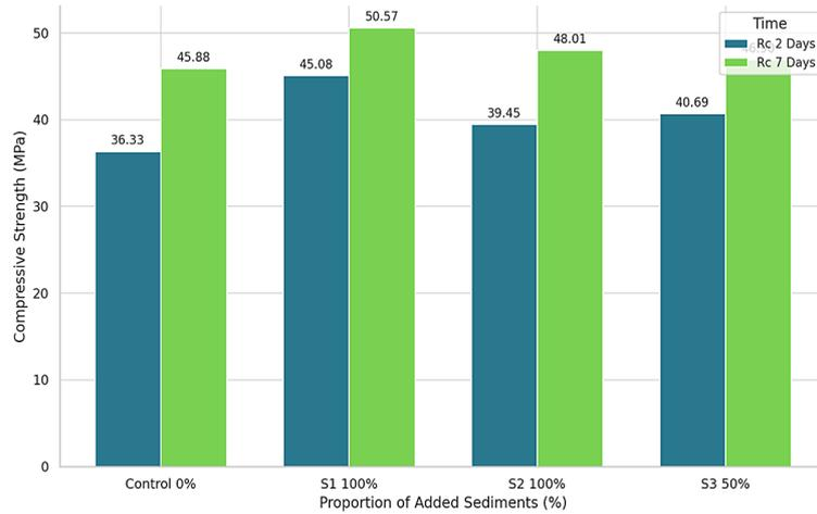
Figure 8. Compressive strength of concrete equivalent mortars (CEMs) with varying substitution ratios of dredged sediments
