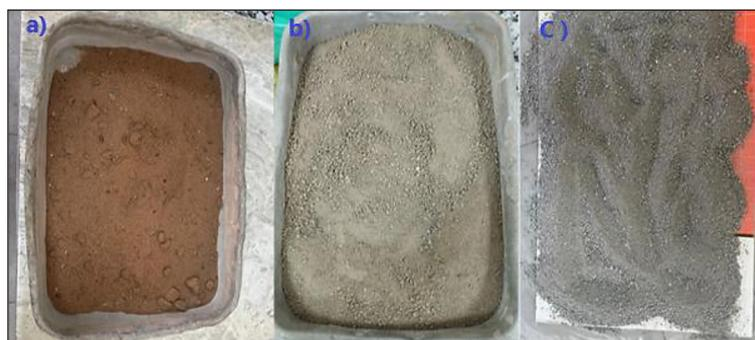
Figure 3. Dune sand (a), dredged sediments (b), and crushed sand (c) used for the formulations
