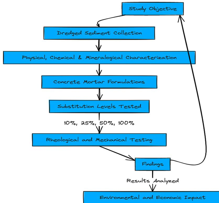
Figure 2. The process of dredged sediment utilization in mortar production
