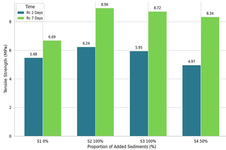
Figure 10. Tensile strength of CEMs with varying substitution ratios of dredged sediments
