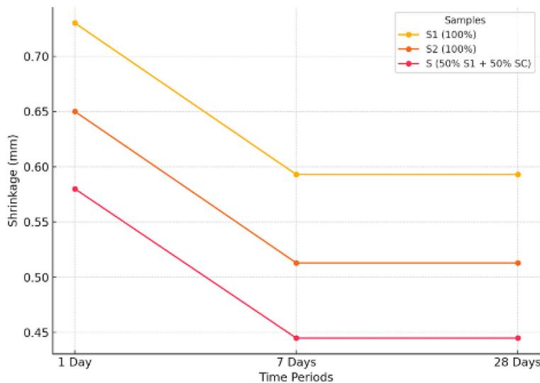
Figure 9. Shrinkage variation over time (1 day, 7 days, and 28 days) for three different samples
