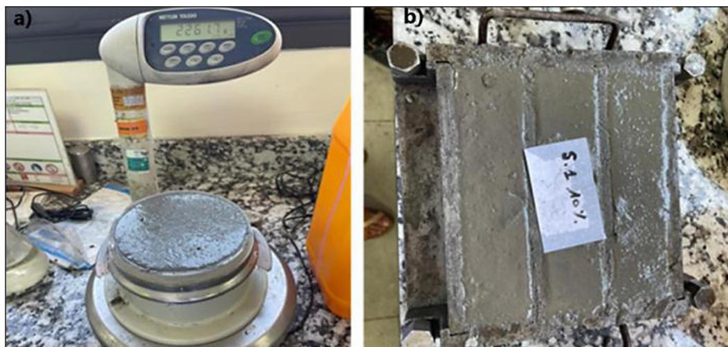
Figure 6. Density measurement (a), and filling of the mini cone using the MBE (b)
