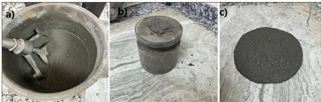
Figure 5. Mixing of concrete in the mixing container (a), filled cylindrical mold for slump flow test (b), spread of concrete after the slump flow test (c)
