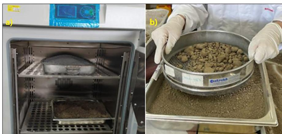
**Figure 4.** Samples dried at 105 °C (a), and sieved through 4 mm mesh sieves (b)
