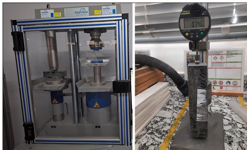
Figure 7. Evaluation of concrete equivalent mortars (CEMs); shrinkage-swelling and compressive strength testing
