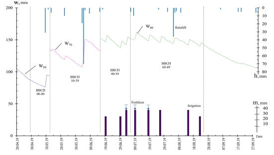
**Figure 2.** Fragmentary hydrograph of soil water reserves with the irrigation regime for grain corn: h – precipitation; m – irrigation rate;  $W_{50-70-80}$  – soil water reserves at depths of 50, 70 and 80 cm, respectively
