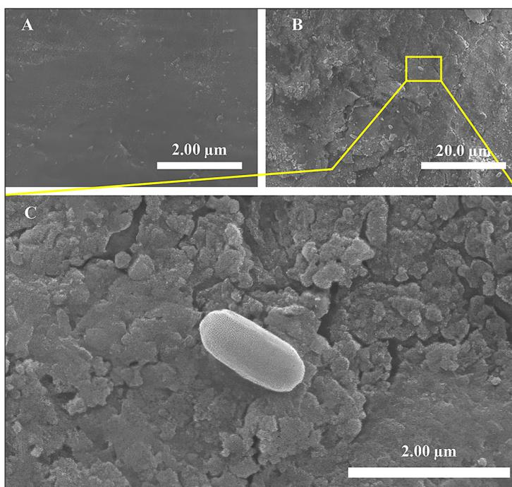
**Figure 6.** Surface morphology of plastics after 30 days of incubation; (a) control (without bacteria); (b, c) are plastics show cracks on the plastic surface by M2
