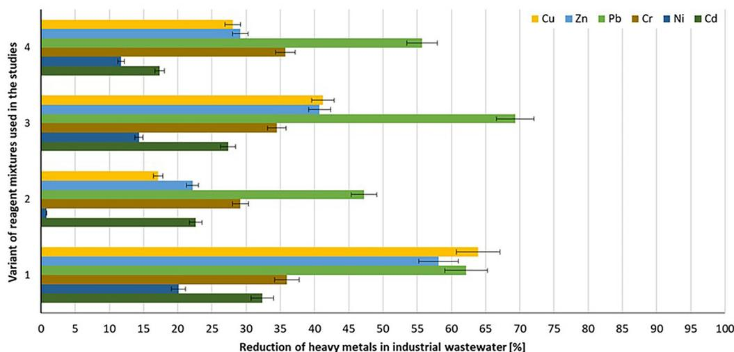
**Figure 1.** Percentage reduction of heavy metal concentration in industrial wastewater for variants 1–4 of the reagent mixtures used
