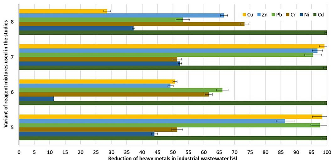
**Figure 2.** Percentage reduction of heavy metal concentrations in industrial wastewater for variants 5–8 of the reagent mixtures used
