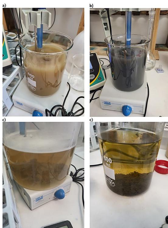
**Figure 3.** Change in colour and turbidity of samples: (a) raw/actual sample, (b) sample after addition of Plexon, (c) sample after addition of Neosorb
