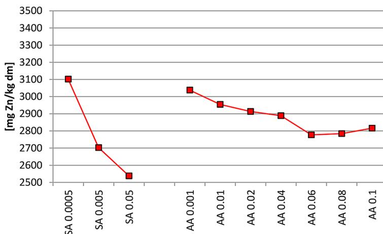
Figure 4. Content of Zn in SSA after extraction
