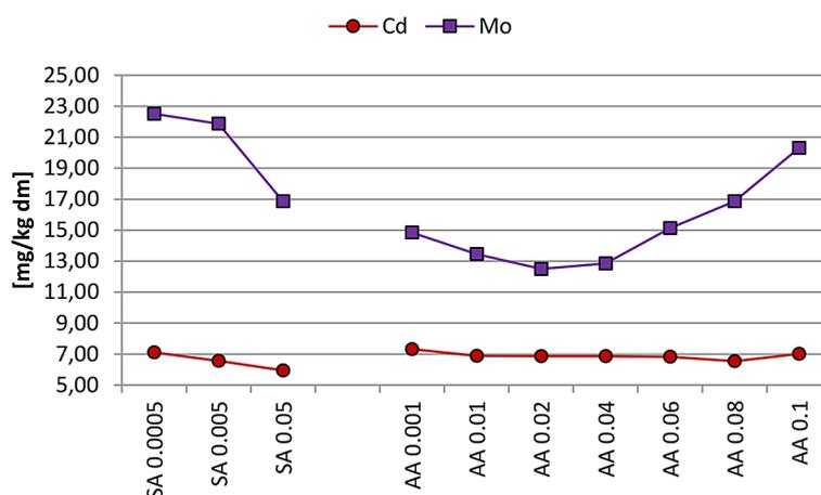
Figure 7. Content of Cd, Mo in SSA after extraction
