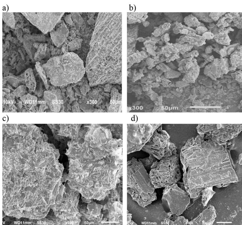
**Figure 5.** SEM analysis of: (a) SRF-Nn+ alginate 0%, (b) SRF-Nn + alginate 2%, (c) SRF-Ni+ alginate 0%, (d) SRF-Ni+ alginate 2%
