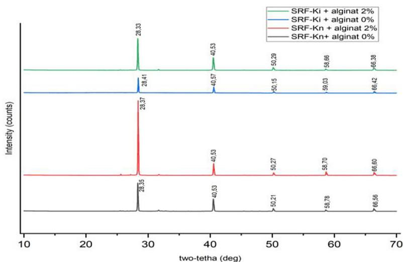
**Figure 9.** XRD analysis of SRF-Kn and SRF-Ki fertilizers with 0% and 2% alginate
