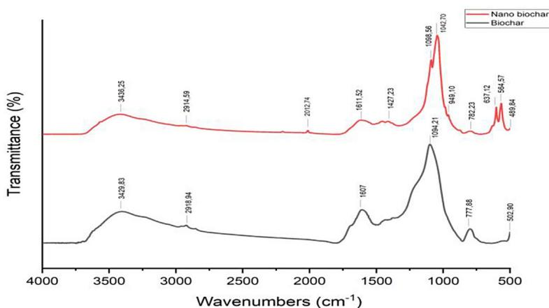
Figure 1. FTIR analysis of biochar and nano biochar
