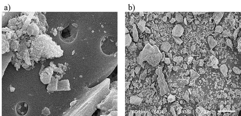
**Figure 4.** SEM analysis results of: (a) biochar, (b) nano biochar
