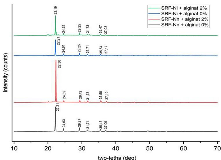
Figure 8. XRD analysis of SRF-Nn and SRF-Ni fertilizers with 0% and 2% alginate
