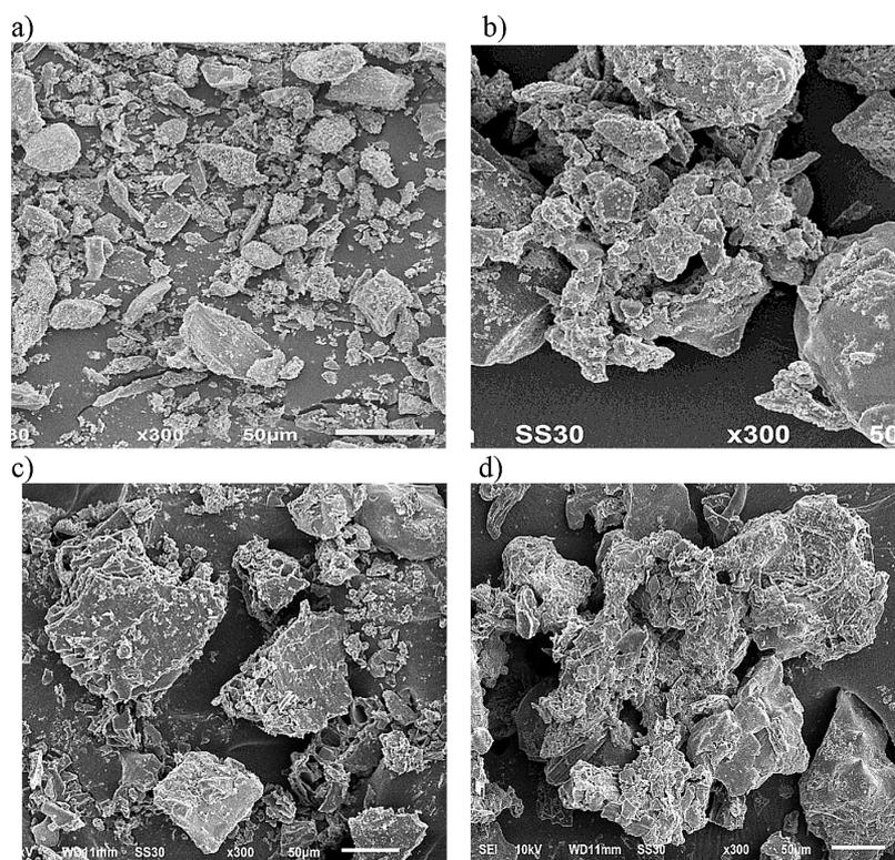
**Figure 6.** SEM analysis results of: (a) SRF-Kn + 0% alginate, (b) SRF-Kn + 2% alginate, (c) SRF-Ki+ alginate 0%, (d) SRF-Ki+ alginate 2%
