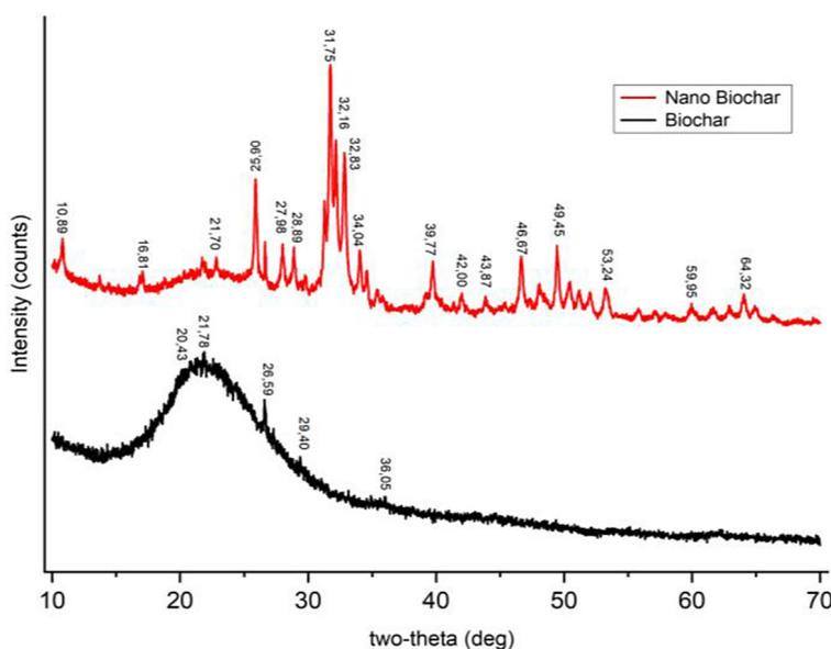
Figure 7. XRD analysis of biochar and nano biochar
