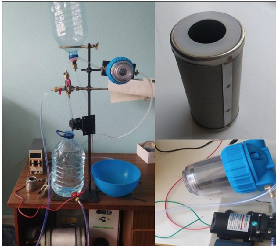
Figure 1. The laboratory setup for filter element research
