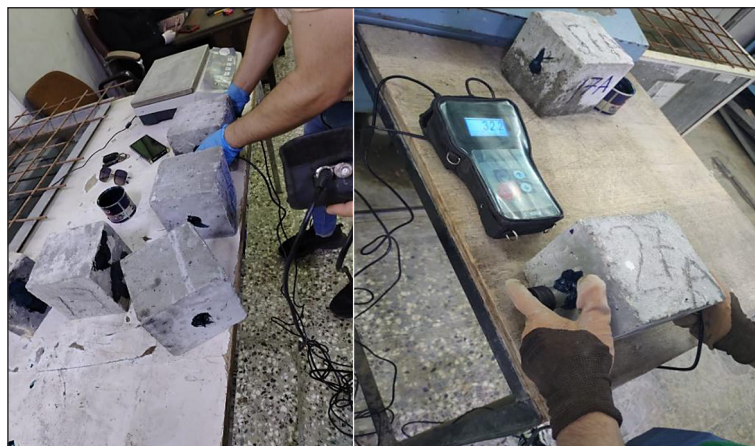
Figure 8. Ultrasonic pulse velocity test
