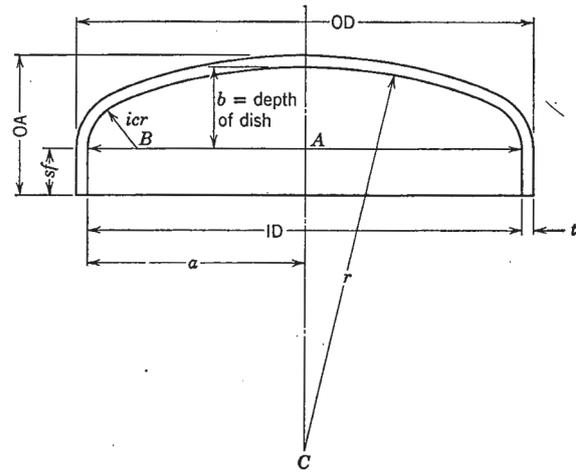
Figure 3. Schematic of torispherical head
