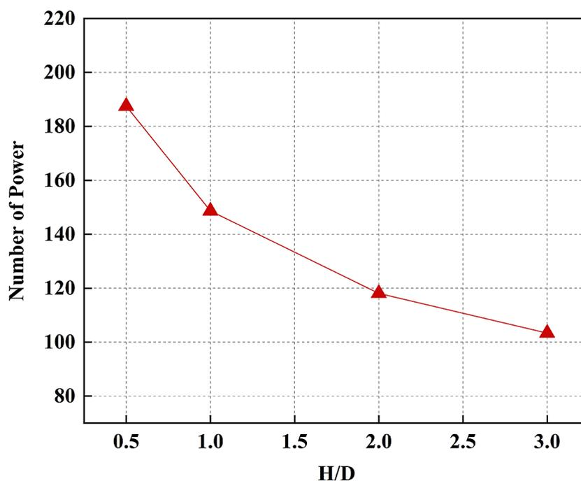
**Figure 4.** H/D ratio vs. number of bioreactor power
