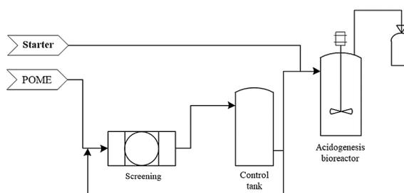
Figure 1. Schematic process of POME acidogenesis
