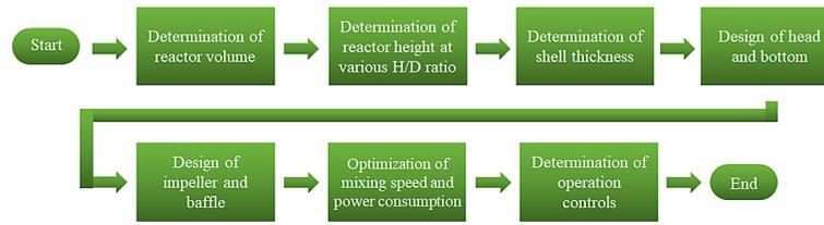
Figure 2. Schematic diagram of bioreactor design
