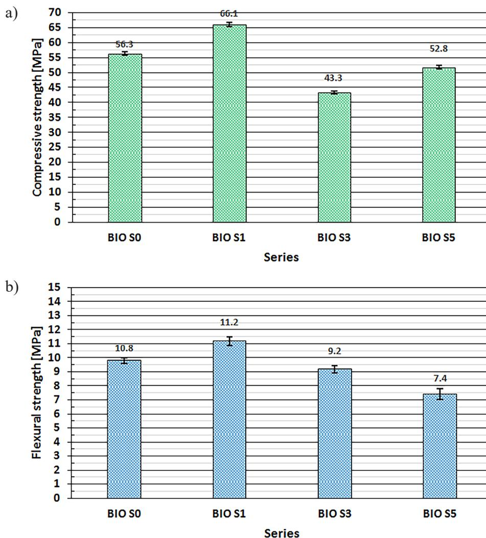
Figure 3. Compressive and flexural strength of mortar with biochar; (a) compressive strength, (b) flexural strength
