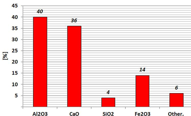
**Figure 1.** Chemical composition of aluminate-calcium cement used in research: Al<sub>2</sub>O<sub>3</sub> – aluminum trioxide, CaO – calcium oxide, SiO<sub>2</sub> – silica dioxide, Fe<sub>2</sub>O<sub>3</sub> – iron trioxide
