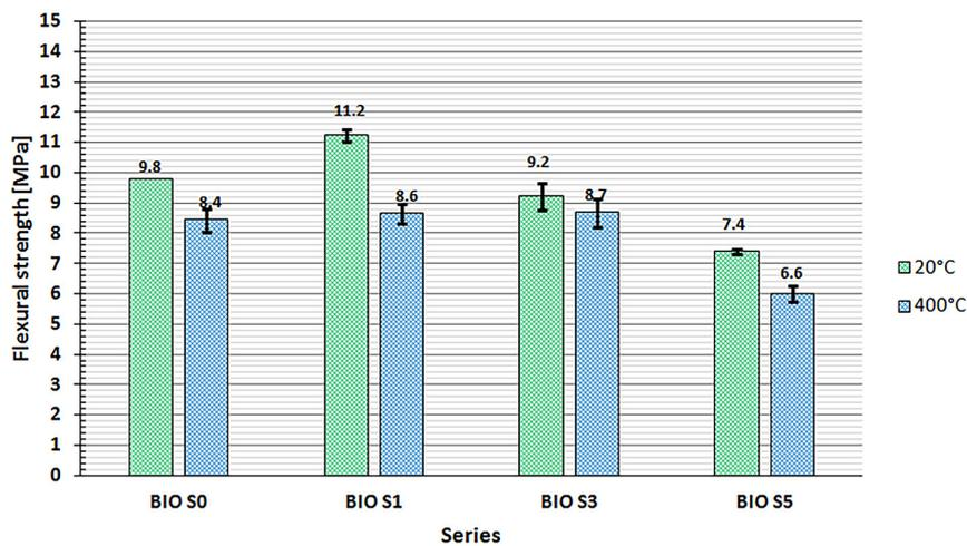
Figure 4. Test results for changes in bending strength after annealing at a temperature of 400 °C
