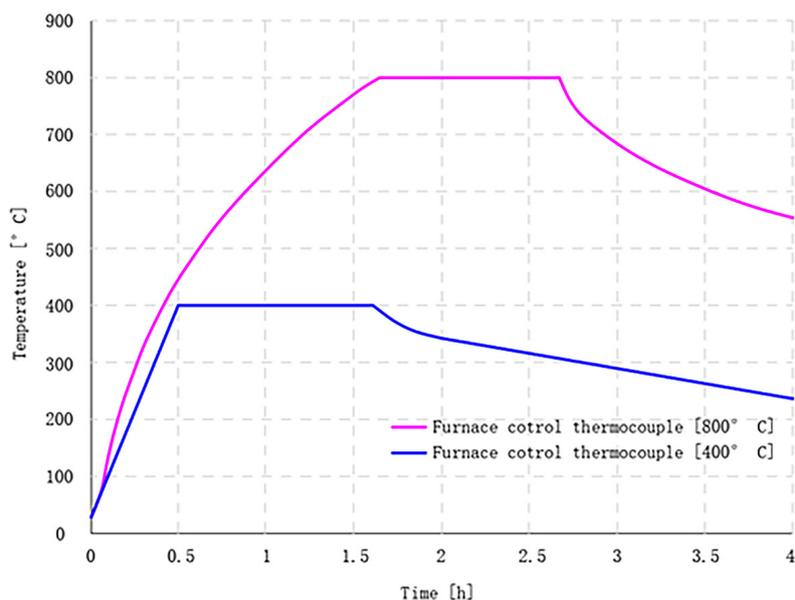
Figure 2. Temperature distribution at 400 °C and 800 °C [PN-EN 1992-1-1]
