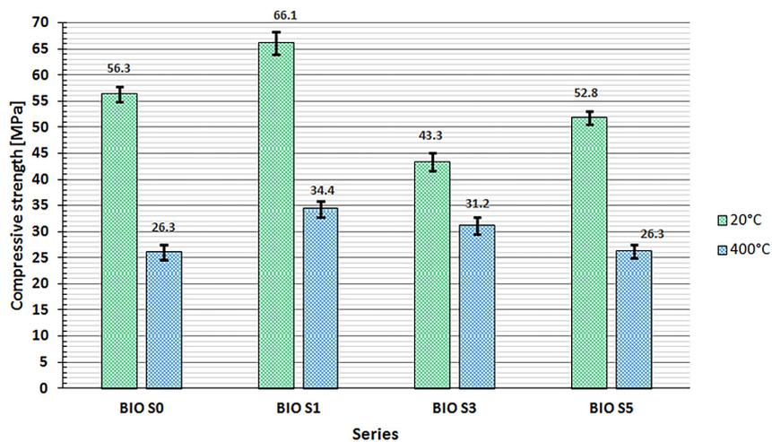
Figure 5. Test results for changes in compressive strength after annealing at a temperature of 400 °C
