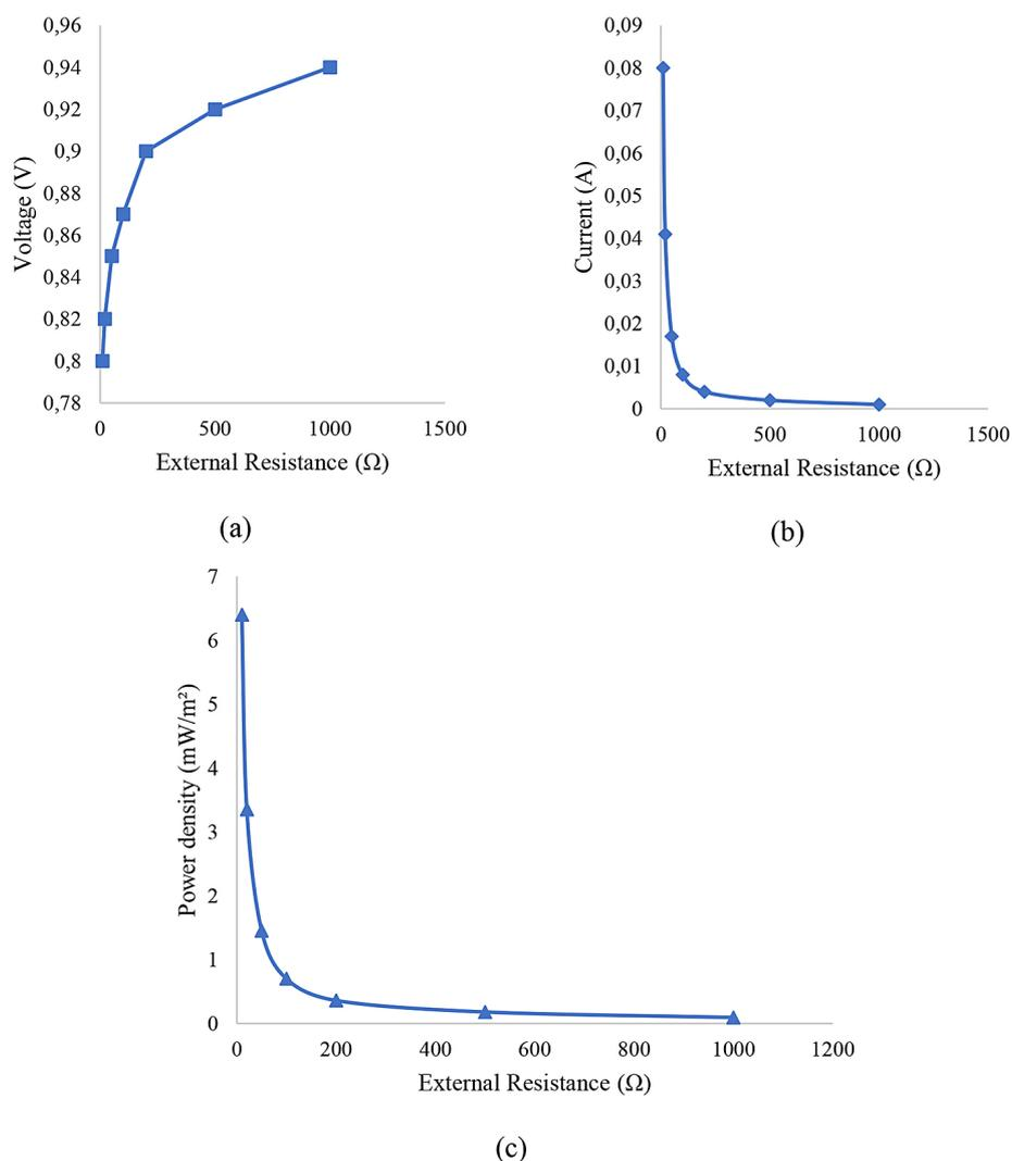
**Figure 2.** Electrochemical performance analysis of the microbial fuel cell (a) polarization curve based on voltage (b) polarization curve: current vs. resistance (c) power curve
