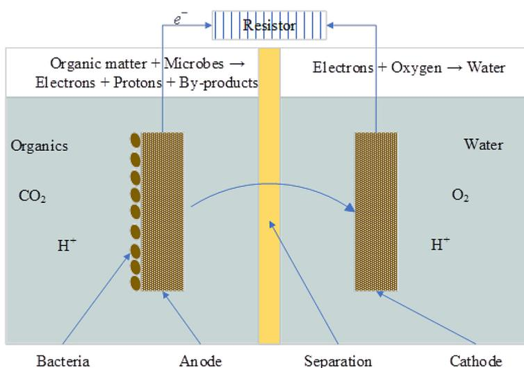
Figure 1. Double chamber MFC setup
