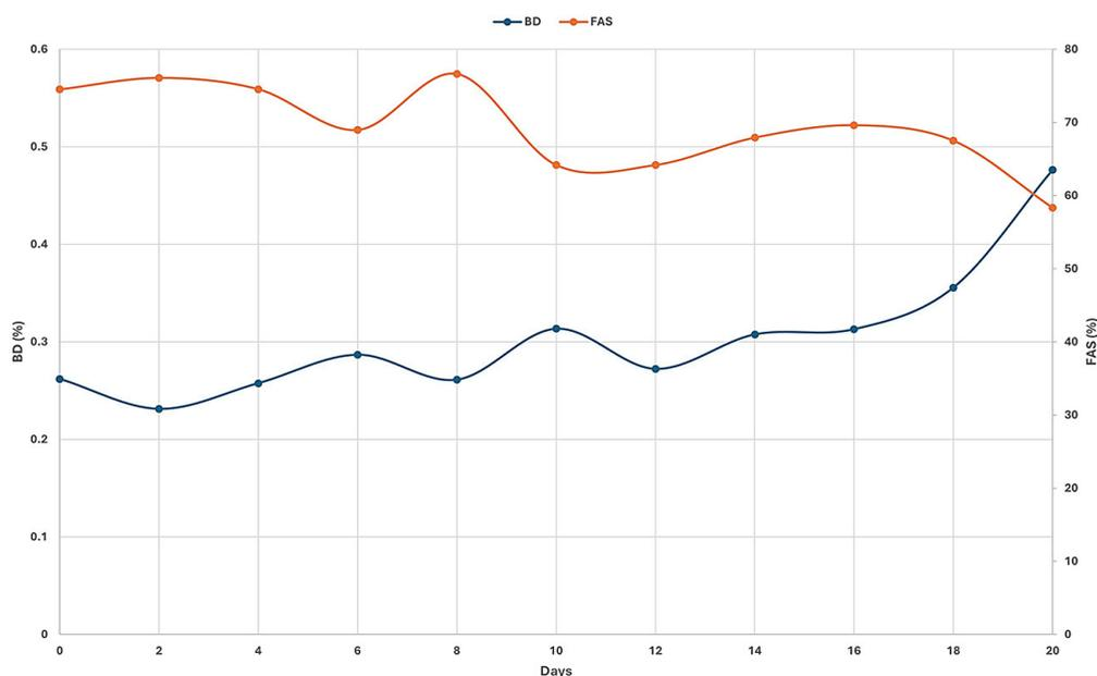
**Figure 4.** The variation in wet Bulk density (BD) and Free air space (FAS) during the composting process
