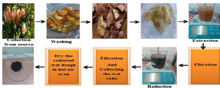
Figure 2. Preparation process of Fe NPS
