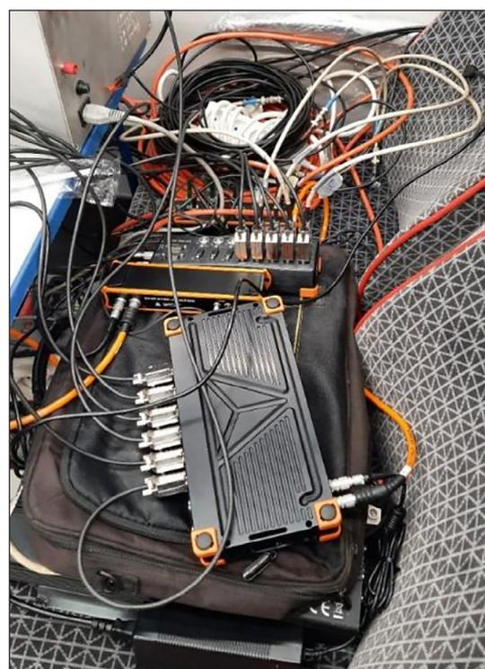
**Figure 2.** SIRIUSie-8xLV+ data acquisition system
