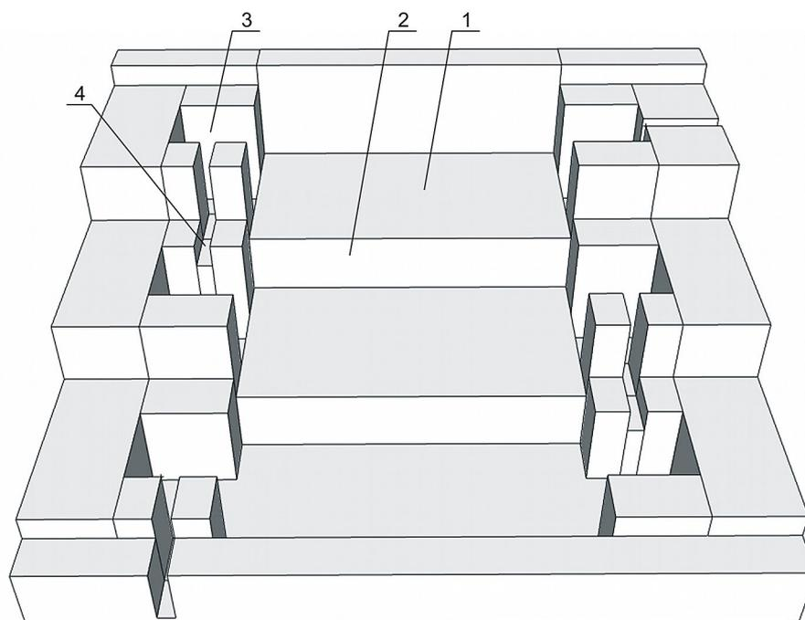
**Figure 8.** PStSF gabion design: 1 – bed box recess, 2 – horizontal base of the bed box, 3 – inspection well recess, 4 – gutter – passage of the pipe connecting the inspection wells
