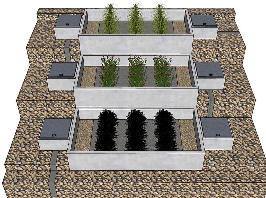
**Figure 10.** An example location of PStSF in the gabion system, including plantings
