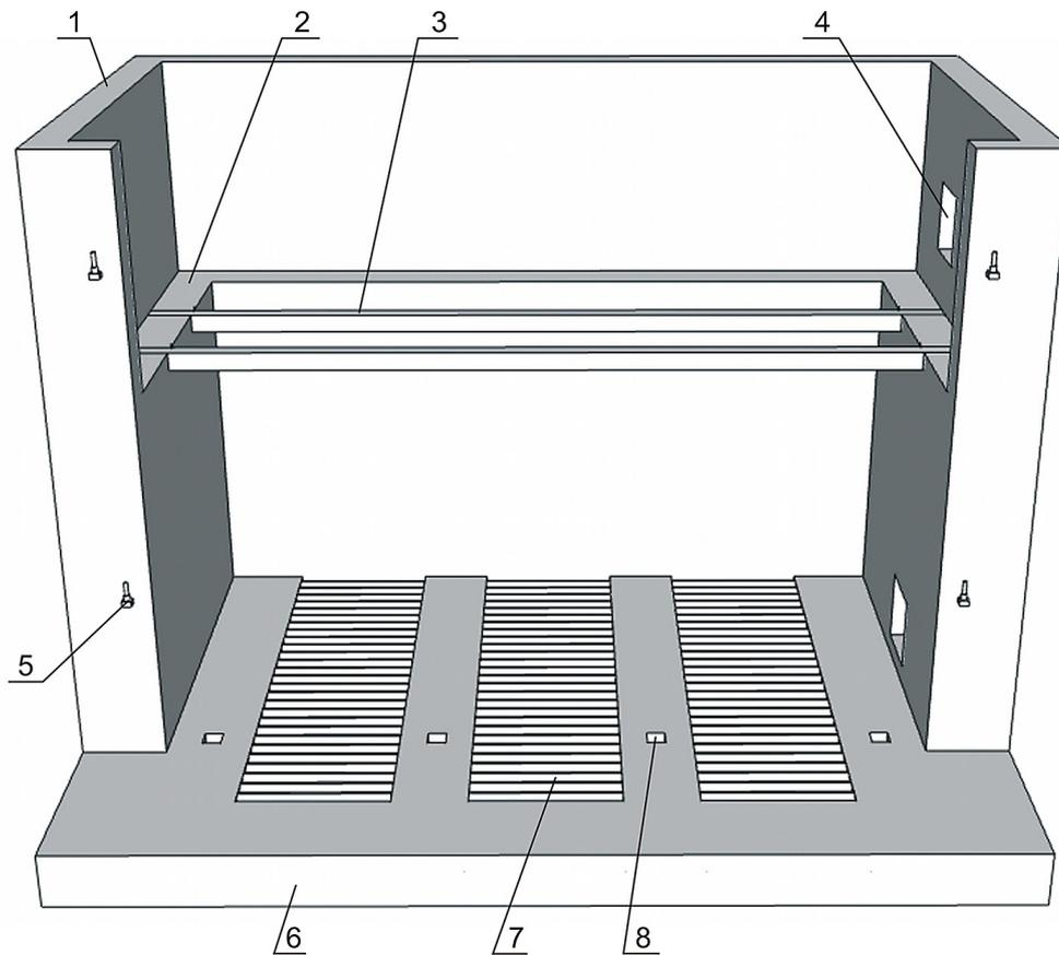
**Figure 5.** PShSF chamber: 1 – vertical wall, 2 – protrusion in the side wall (internal step) – upper bed support, 3 – longitudinal beam – upper bed support, 4 – hole (pipe passage), 5 – hinge for mounting technical doors, 6 – horizontal base (bottom/foundation plate), 7 – gutter with a set of rollers – support of the lower bed, 8 – hole for the retaining wedge
