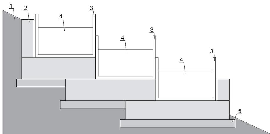
**Figure 9.** PStSF with elements of anti-erosion protection (side view): 1 – ground, 2 – supporting structure (gabion casing), 3 – bed box, 4 – planted soil bed, 5 – base (e.g. strip footing)
