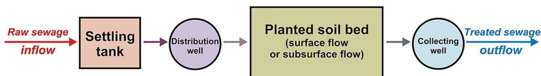
**Figure 1.** Layout of a wetland wastewater treatment plant with a planted soil bed
