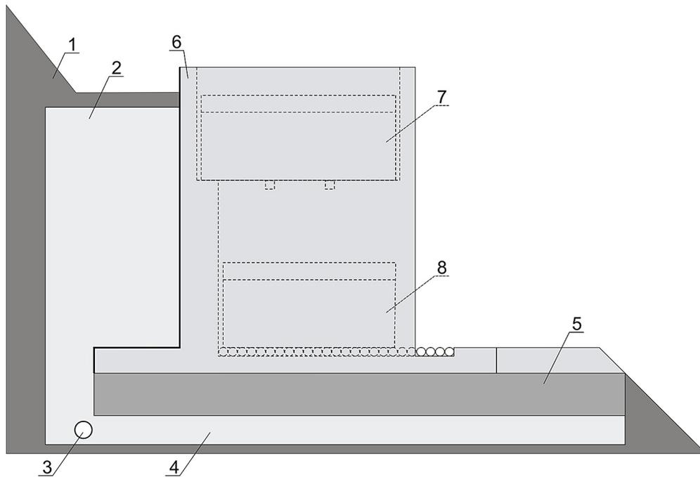
**Figure 4.** PShSF with elements of anti-erosion protection (side view): 1 – ground, 2 – filling (e.g. crushed stone), 3 – drainage, 4 – frost-proof layer (e.g. crushed stone), 5 – foundation, 6 – shelf filter chamber, 7 – upper box, 8 – lower box
