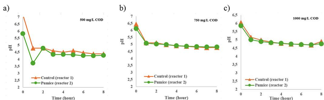
**Figure 5.** Comparison of changes in pH in the tripikon-S reactor 1 (control) and reactor 2 (pumice) in the first 8 hours of treatment at COD doses (a) 500 mg/L; (b) 750 mg/l and (c) 1000 mg/l
