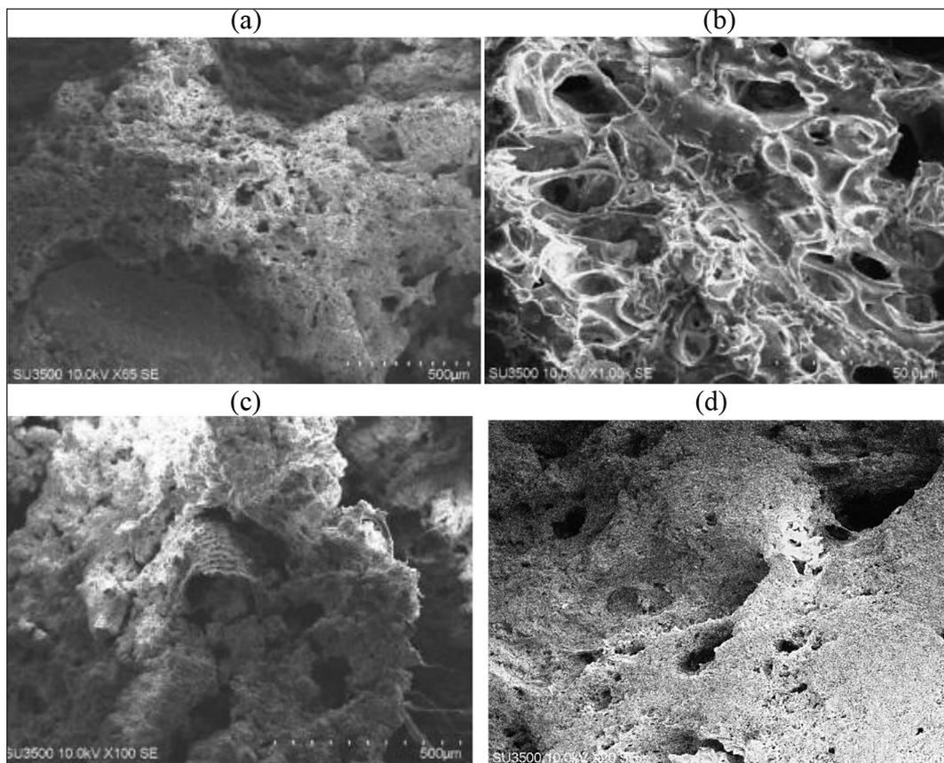
**Figure 8.** Biofilm surface on pumice observed using SEM microscope on (a) day 0; (b) day 108; (c) day 151; (d) day 162
