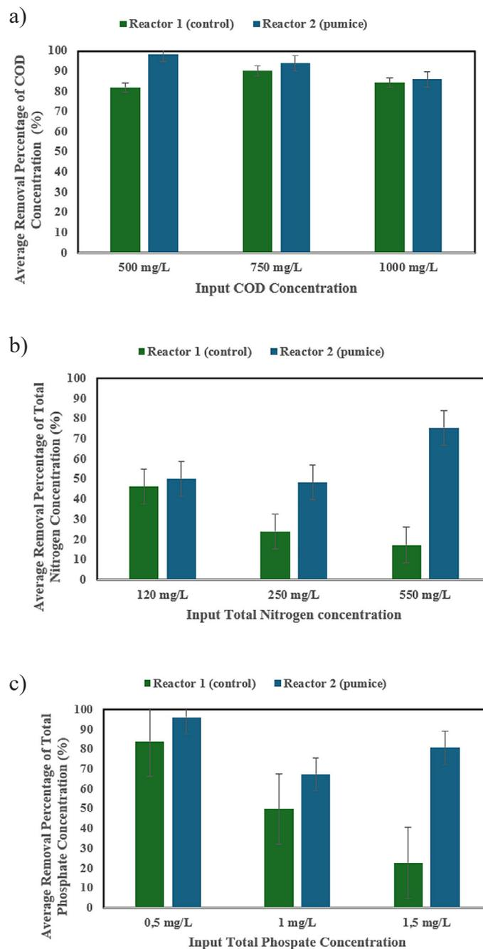
**Figure 6.** Comparison of average concentration of removal of (a) COD, (b) total nitrogen and (c) total phosphate in tripikon-S between reactor 1 (control) and reactor 2 (pumice)
