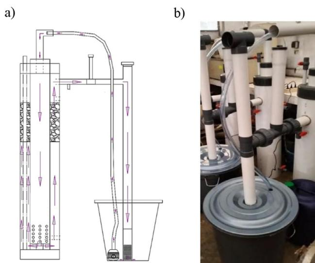
**Figure 2.** (a) Design of operational settings and (b) existing conditions of the reactor when operated
