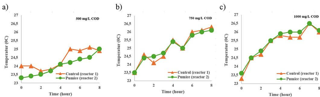
Figure 3. Comparison of changes in temperature in the tripikon-S reactor 1 (control) and reactor 2 (pumice) in the first 8 hours of treatment at COD doses (a) 500 mg/L; (b) 750 mg/l and (c) 1000 mg/l
