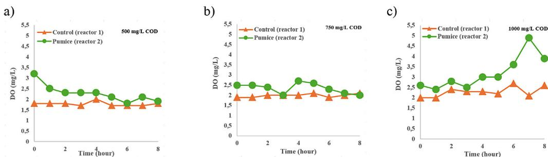
Figure 4. Comparison of changes in DO in tripikon-S reactor 1 (control) and reactor 2 (pumice) in the first 8 hours of treatment at COD doses (a) 500 mg/L; (b) 750 mg/l and (c) 1000 mg/l
