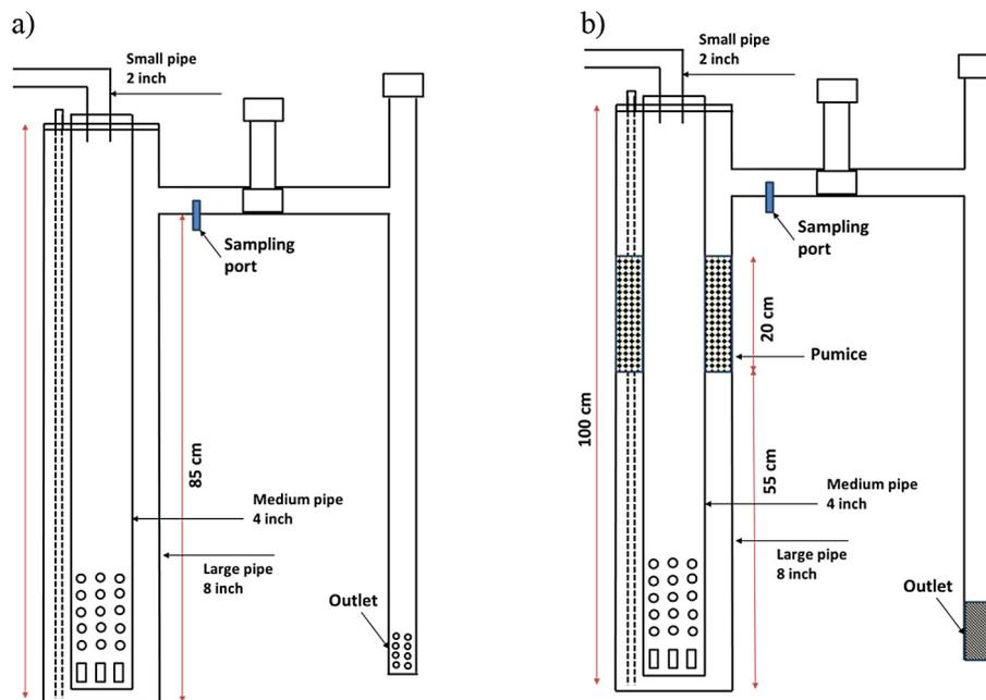
Figure 1. Design of tripikon-S (a) reactor 1 without modification and (b) reactor 2 modified pumice and fiber filter
