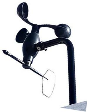
Figure 1. Anemometer used to measure wind speed and direction
