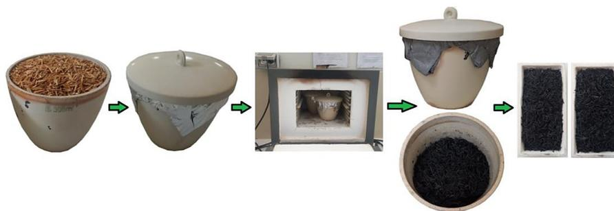
Figure 1. Preparation of biochar derived from rice husks
