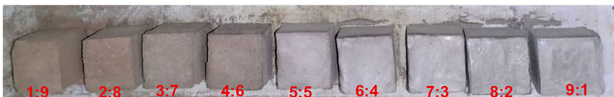
Figure 3. Comparison of compressive strength with cement usage in test specimens (a) STTG (b) SSTG (c) STG with dimensions of 5 \times 5 \times 5 cm
