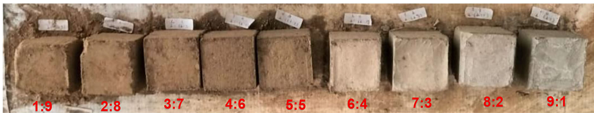
(a) Cement + Tanah Tras : Tailing (STTG)
