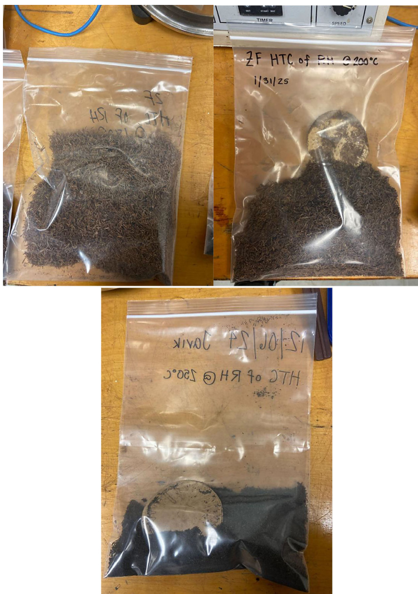
Figure 3. Rice husks after HTC treatment at 180 °C (left top), 200 °C (right top), and 250 °C (bottom)
