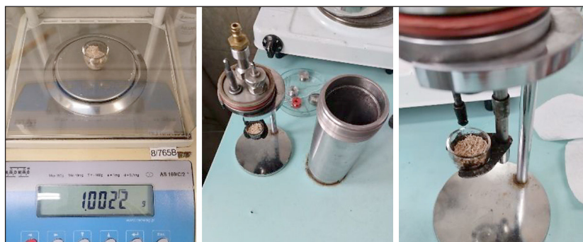
Figure 3. A calorimetric method for calorific value determination
