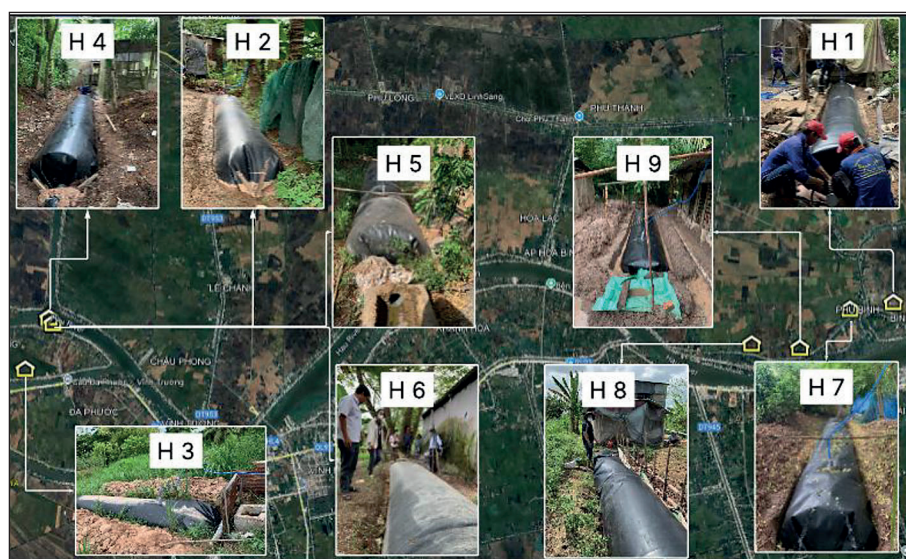
Figure 1. Installed sites of nine HDPE biogas digesters
