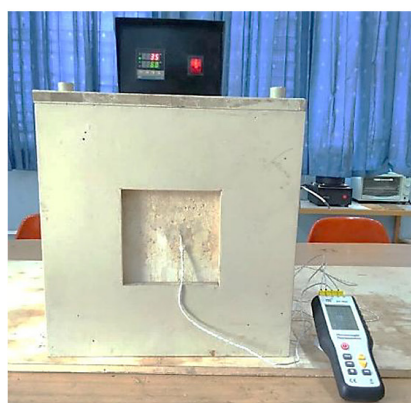
Figure 4. Insulation box for measuring the thermal conductivity of PUR composites
