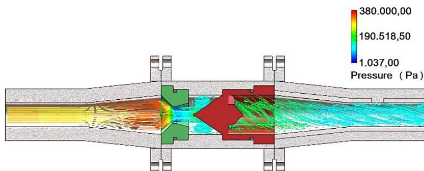
Figure 3. Cavitation reactor CAV-V – cross section
