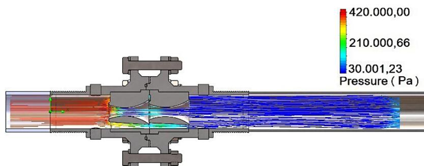
Figure 2. Cavitation reactor CAV-2A – cross section
