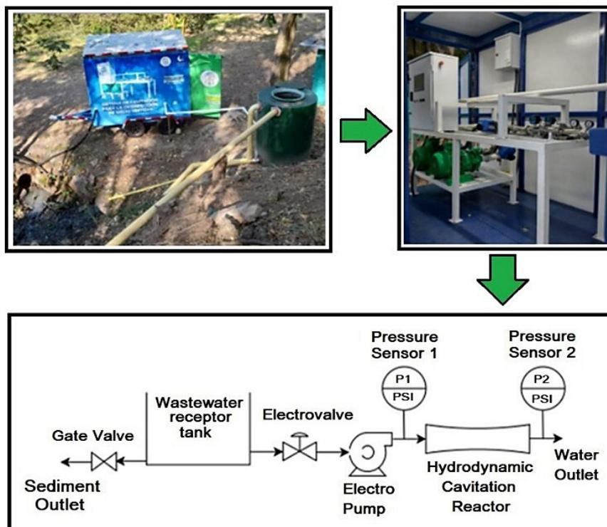
Figure 4. HC system schematic
