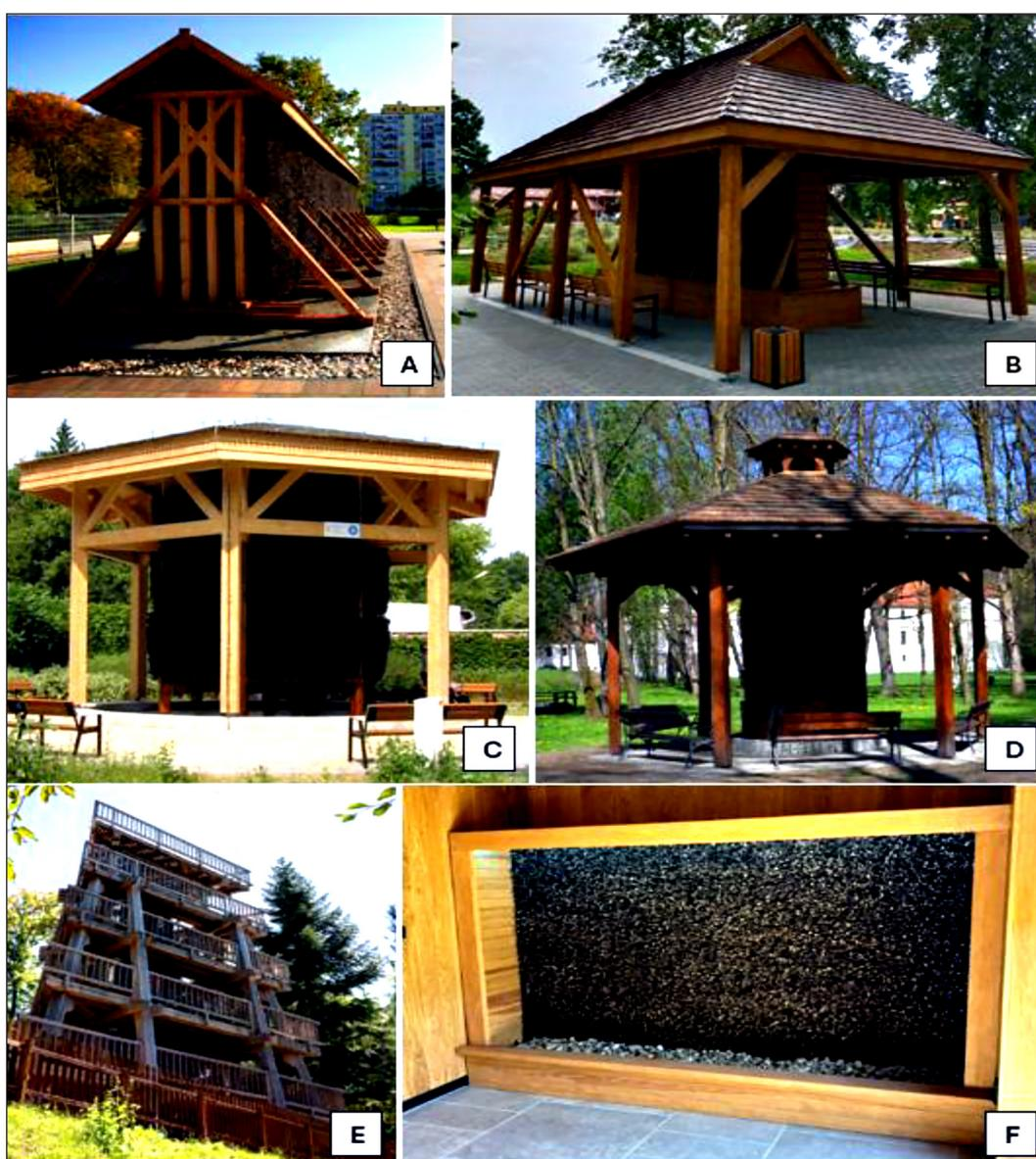
**Figure 3.** Architectural forms of brine graduation towers: A – longitudinal, B – longitudinal with a roof for visitors, C – central, D – central with a roof for visitors, E – observation tower, F – facade (<https://zsm.lodz.pl>; <https://aranzacjekopalniane.pl>; <https://www.twoja-praga.pl>; <https://sucha-beskidzka.pl>; <https://turystyka.glucholazy.pl>; <https://dorako.pl>)
