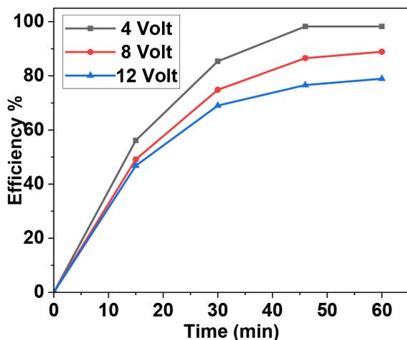
Figure 2. Effect of voltage on lowering mercury levels
