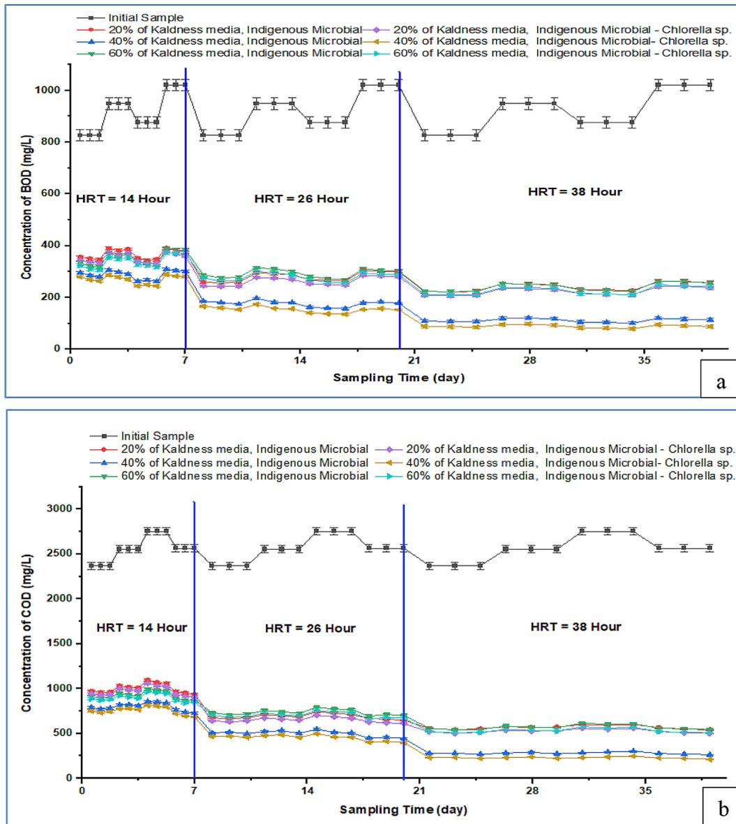
Figure 2. Effect of hydraulic retention time (HRT) on BOD<sub>5</sub> (a) and COD (b) removal efficiency in microbial and algal biofilm systems. Data represent mean ± SD (n = 7)
