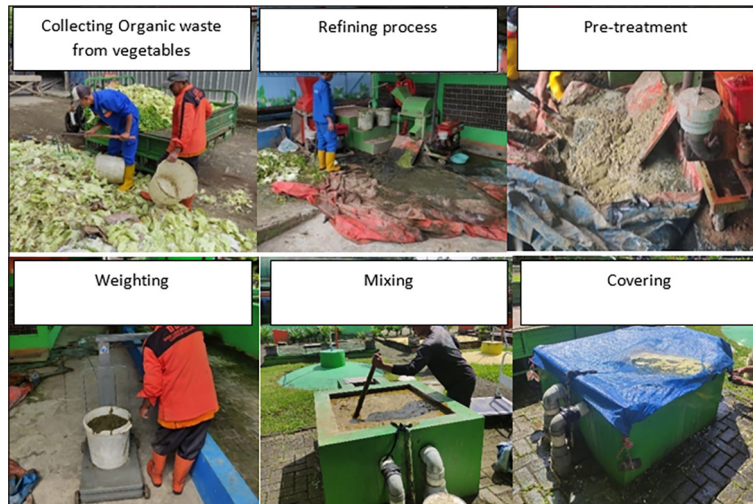
Figure 2. Process of producing methane gas in IRRC
