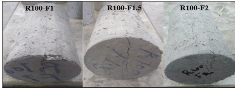
Figure 10. The failure mode of splitting tensile strength specimens with R=100% and various ratio of Vf %
