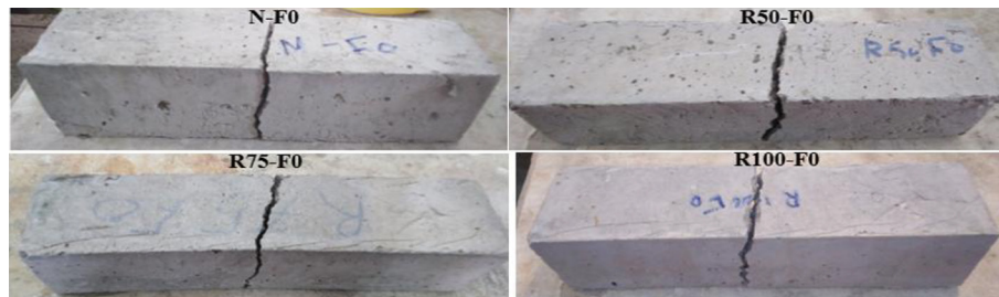
Figure 8. The failure mode of specimens for flexural strength with various ratio of R%
