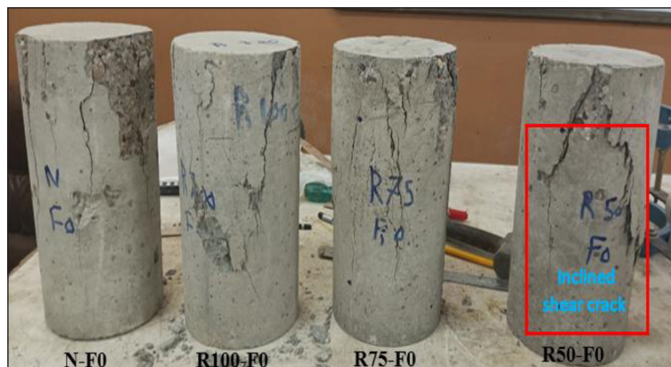
Figure 6. Cylindrical specimens after a compression test with different ratios of R%
