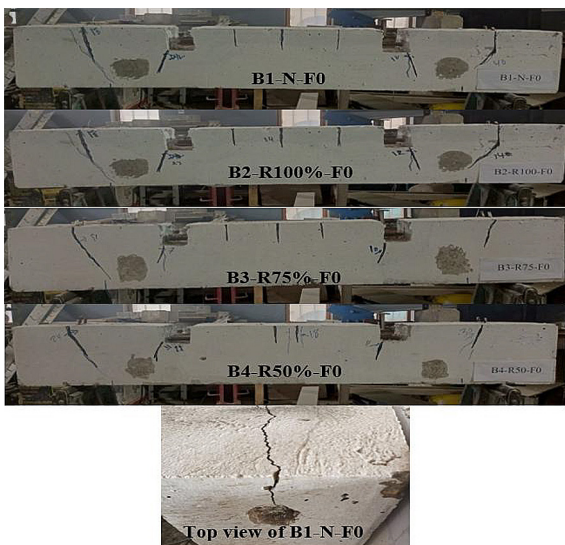
Figure 12. Examined beams from group 1, as well as the control beam (B1-N-F0)
