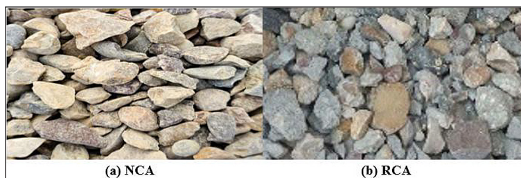
Figure 1. Several types of coarse aggregates that were utilized in this investigation (a) NCA, (b) RCA
