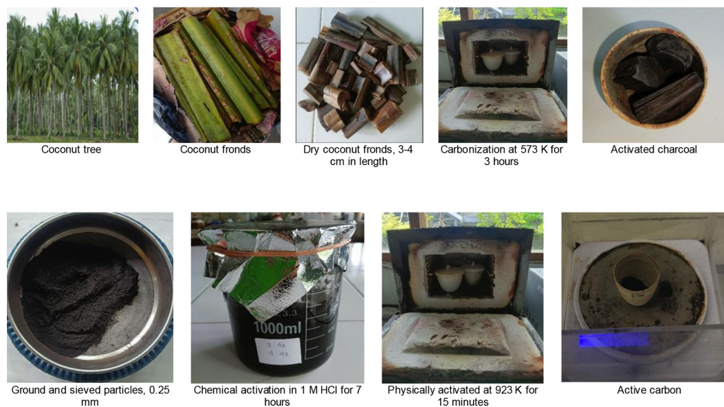
Figure 1. Preparation of activated carbon from coconut fronds
