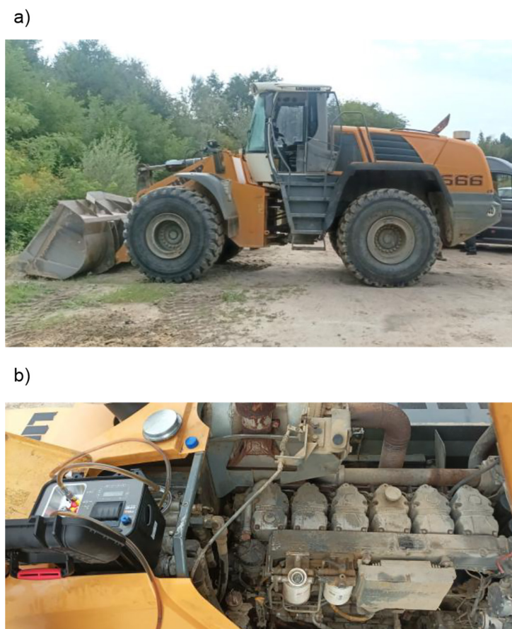
Figure 2. View of: a) the Liebherr 566 wheel loader used in the experiments, b) oil cleanliness class testing using an ArgoHytos analyzer
