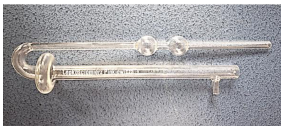
Figure 4. View of: a) preparation of the capillary for kinematic viscosity measurement, b) Ostwald–Pinkiewicz capillary with a constant k = 0.2736
