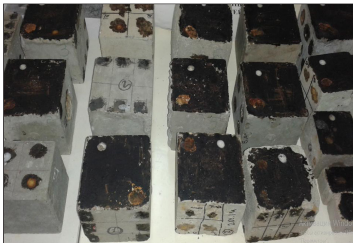
Figure 1. Various grades of concrete contaminated with fuel oil under model conditions
