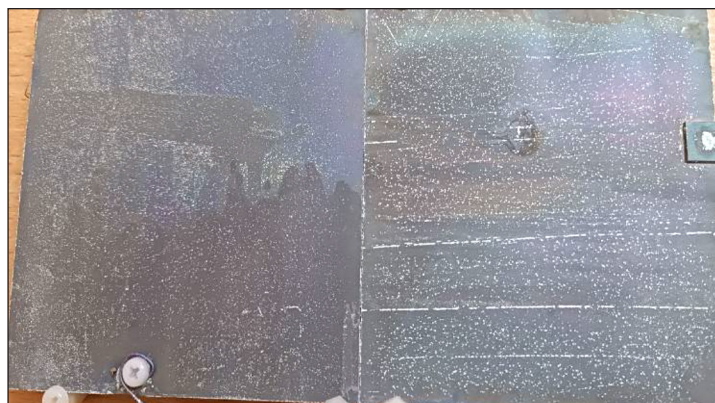
Figure 6. Traces of corrosion (TiO 2 ) on a titanium anode with a ruthenium oxide coating
