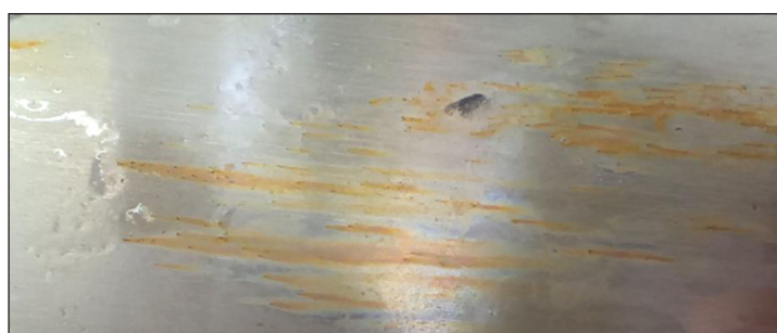
Figure 5. Traces of pitting corrosion on a stainless steel electrode
