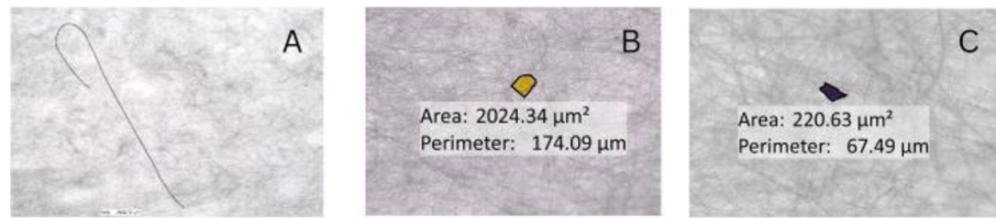
Figure 5. Representative microplastic types observed at the sampling sites: (a) fiber, (b) film, and (c) fragment
