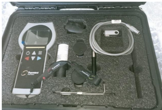
Figure 3. Thermtest TLS-100 conductivity and thermal resistance measurement equipment
