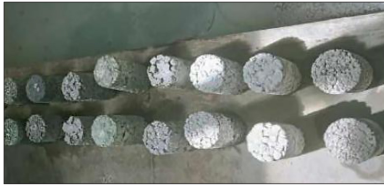
Figure 2. View of the permeable concrete test tubes designed in this study
