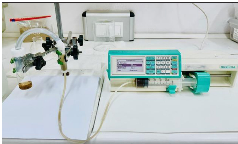
Figure 2. Experimental setup for sorption testing using a Medima S1 infusion pump
