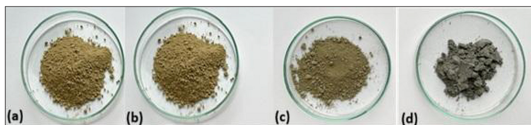
Figure 1. Samples of studied substrates: (a) Chotyłów, (b) Chotyłów with addition of 10% NaP1 zeolite, (c) Chotyłów with addition of 20% NaP1 zeolite, and (d) NaP1 zeolite
