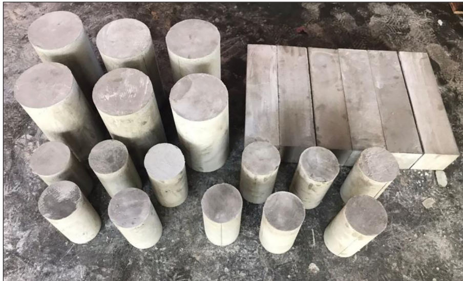
Figure 5. Preparation of foamed concrete specimens
