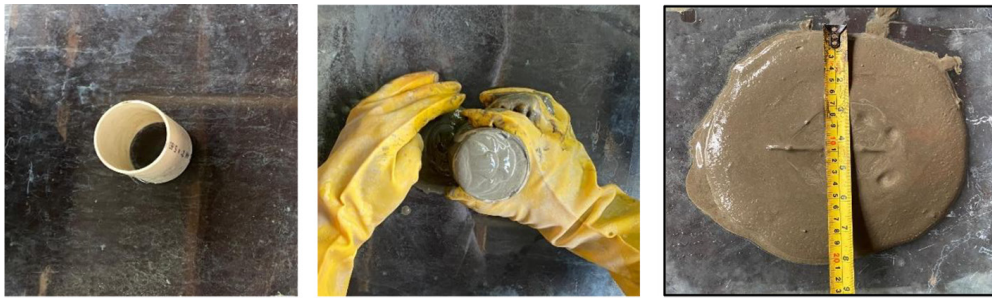
Figure 7. Slump flow testing procedure
