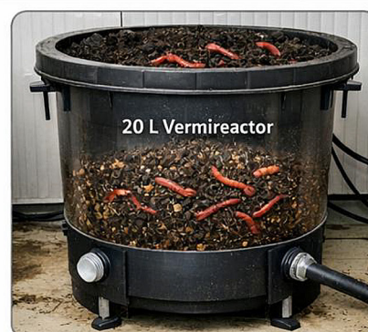
Figure 1. Experimental workflow and laboratory-scale vermireactor setup: (a) stepwise workflow from raw material preparation to vermicomposting and sample analysis, highlighting key parameters: substrate C/N ratio, moisture content, brown coal addition, and earthworm density/biomass; (b) laboratory-scale 20 L vermireactor with Eisenia fetida , illustrating feeding, weekly mixing, and aeration setup
