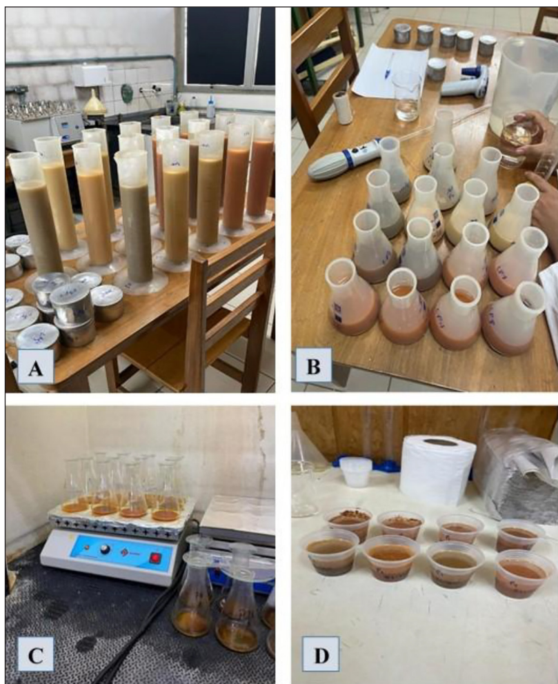
Figure 3. Soil samples being processed for the determination of soil texture (A) and (B); (C) samples being processed for organic matter determination; and (D) samples in water for pH determination
