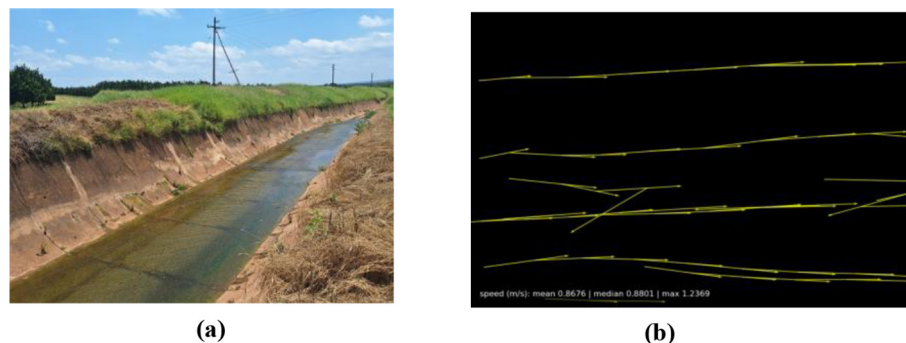
Figure 6. Case Study 2 measurement site and results, showing (a) the measurement location and (b) the corresponding velocity vector field
