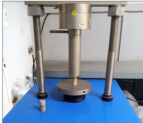
Figure 4. Compressive strength test of CEBs
