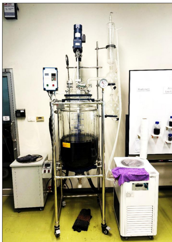
Figure 1. Hydrometallurgical reactor setup used for metal recovery from lithium-ion battery black mass
