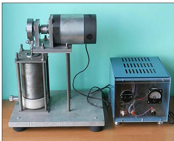
Figure 1. The general appearance of the piston type vibration cavitator
