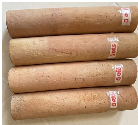
Figure 1. Photographic appearance rice husk-derived low-cost ceramic membrane
