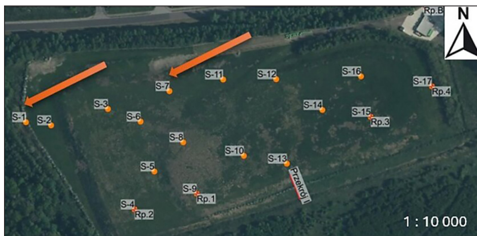
Figure 3. Location of the vertical degassing well for determining the landfill gas composition at site A (50°48'51.40" N; 16°18'36.55" E, administrator's archive materials)
