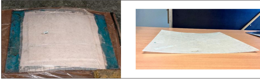
Figure 2. Fabricated GFRP cylindrical shell structure
