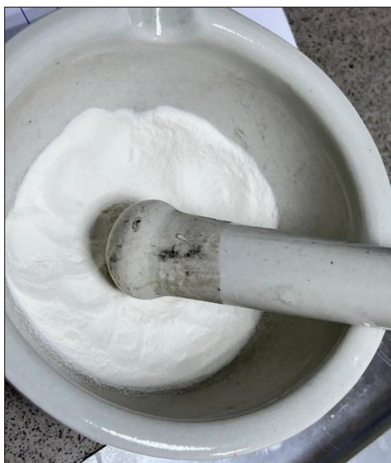
Figure 1. Manual grinding of dried CMC powder using a porcelain mortar and pestle as a preliminary size-reduction step prior to mechanical milling
