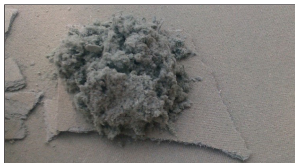
Fig. 2. Crushed waste underlay boards under floor panels
