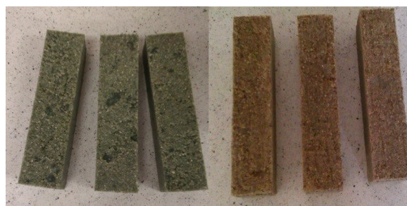
Fig. 8. The appearance of samples before and after the test of freezing resistance
