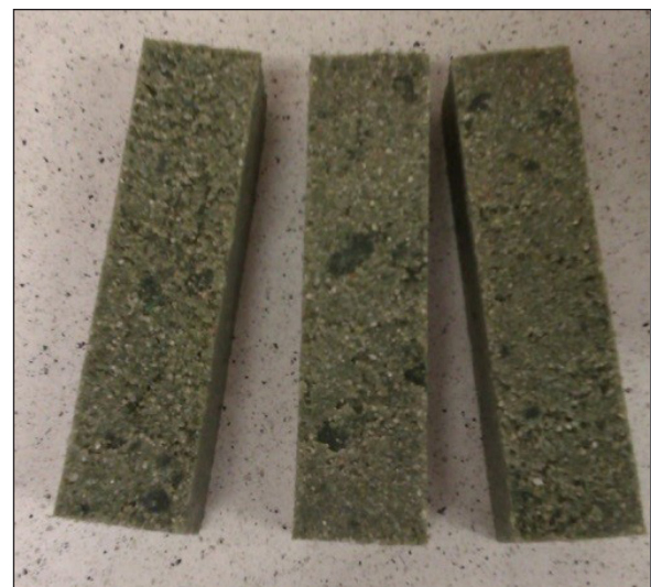
Fig. 3. Samples intended for endurance tests with 35-percent waste board wood
