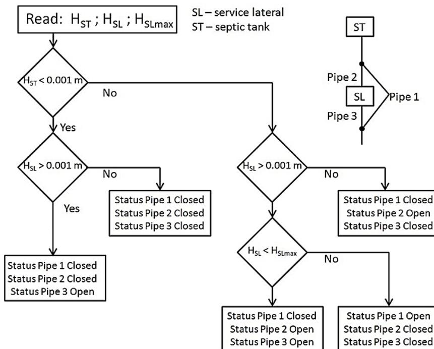
Figure 9. Block diagram of the opening and closing of bypass simulating service lateral
