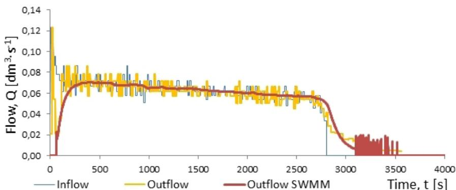
**Figure 13.** Inflow and outflow rates from the installation during emptying the tank as in Figure 5, measured (step-wise line) and generated by model C
