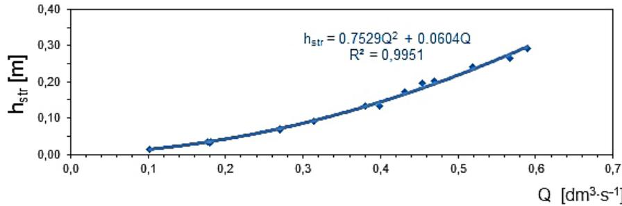
Figure 7. Pressure loss in float-ball valve with seats of diameter 25 mm depending on flow rate [Nawrot 2011]
