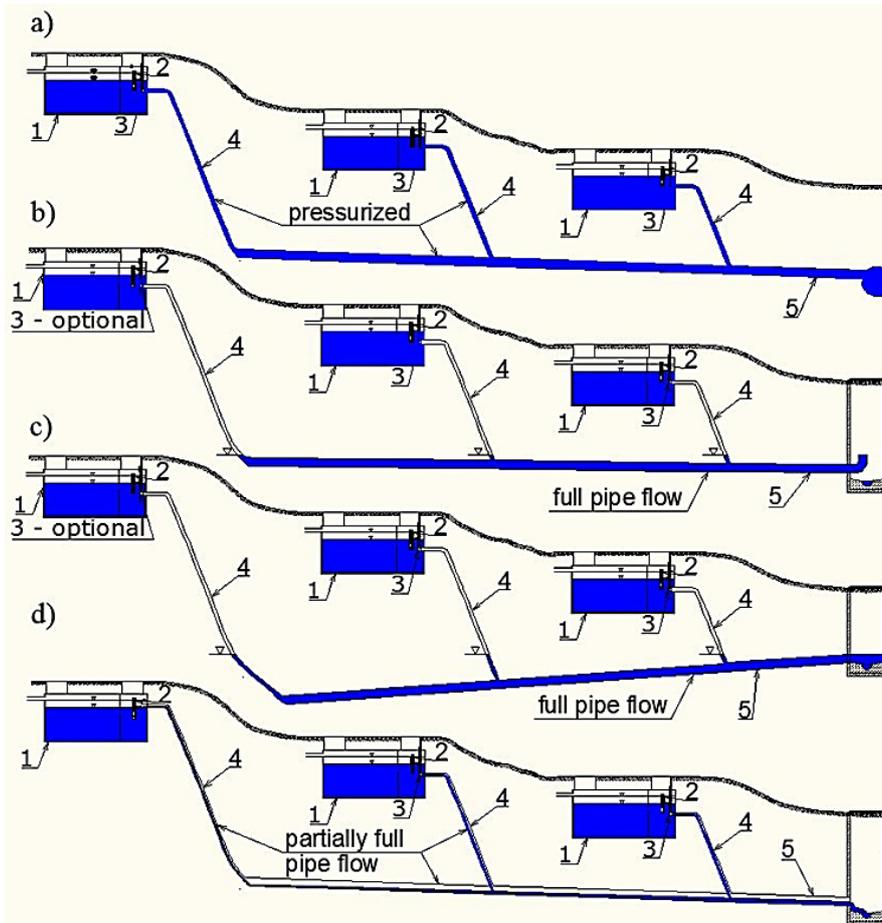
**Figure 5.** Hydraulic schemes of SDGSS: a) pressurized system simulated in EPANET 2.0 as model A, b-c) surcharged systems simulated in EPANET 2.0 as model B, d) free-water-surface system simulated in SWMM 5.0 as model C; Legend: 1 – septic tank, 2 – effluent screen filter, 3 – float-ball valve, 4 – service lateral, 5 – collection main
