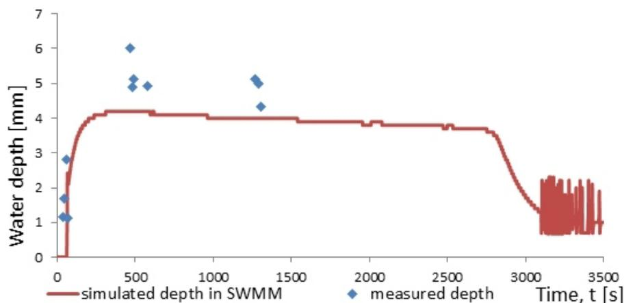
**Figure 14.** Water depth measured at the outlet of the experimental set-up as in Figure 5 and simulated by model C
