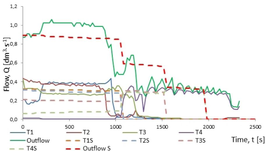
**Figure 11.** Outflow rates from the tanks and installation during simultaneous emptying, measured (solid lines) and generated (dashed lines) by the model A
