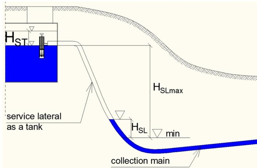
Figure 8. Sketch diagram of model B showing wastewater outflow from ST and service lateral simulated as a tank
