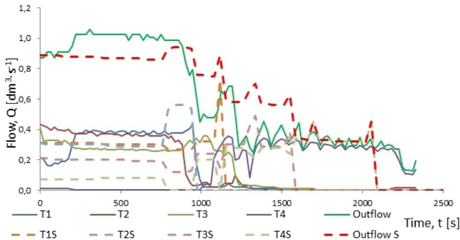
**Figure 12.** Outflow rates from the tanks and installation during simultaneous emptying, measured (solid lines) and generated (dashed lines) by the model B
