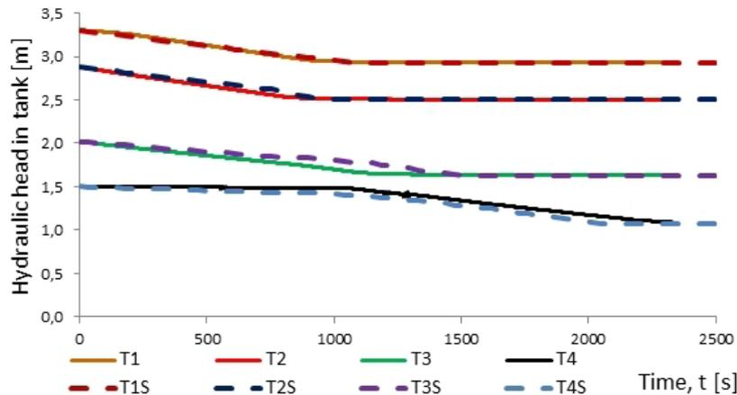
**Figure 10.** Measured (solid lines) and generated by the model A (dashed lines) hydraulic heads in tanks during their simultaneous emptying
