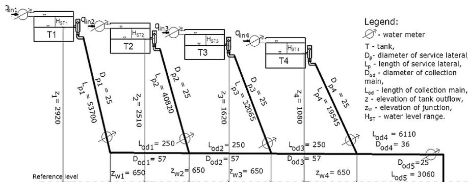
Figure 2. Layout of the laboratory installation (all dimensions in mm)
