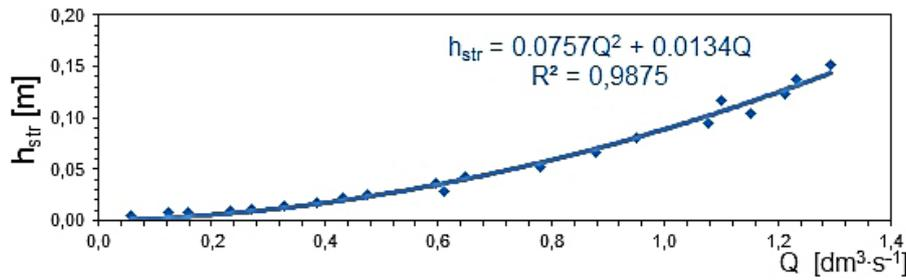
Figure 6. Pressure loss in effluent screen filter depending on flow rate [Nawrot 2011]
