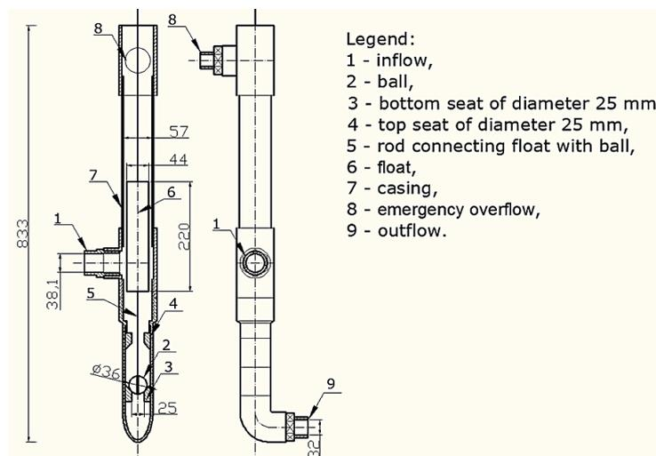
Figure 3. Vertical cross section and side view of float-ball valve (dimensions in mm)
