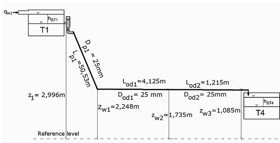
Figure 4. Scheme of installation used to verify the model implemented in the SWMM
